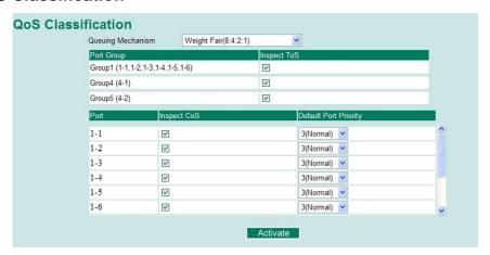
The PT-7728 supports inspection of layer 3 TOS and/or layer 2 CoS tag information to determine how to classify traffic packets.
